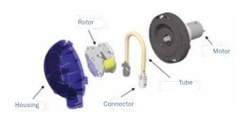
The transport volume depends on the speed, number of rollers and the diameter of the transport tube. The elasticity of the tube is sufficient to generate the required negative inlet pressure. The maximum pressure is generally 1 bar.
